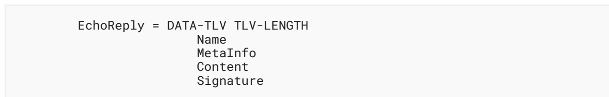
Figure 8: Echo Reply NDN Packet Format
