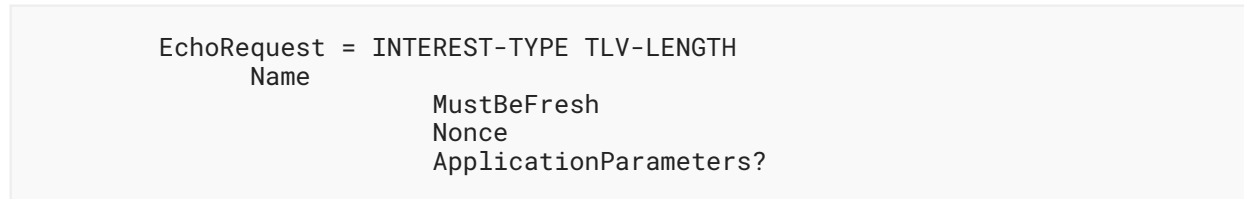
Figure 7: Echo Request NDN Packet Format
